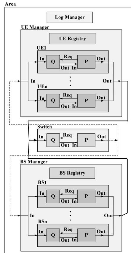
Figure 4. Simplified DEVS model hierarchy for mobile network model (Q: Queue, P: Processor)
