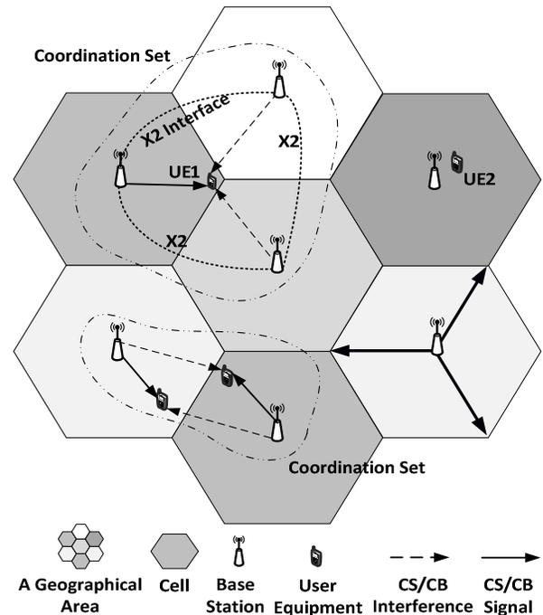
Figure 1. CS/CB transmission in LTE-Advanced
