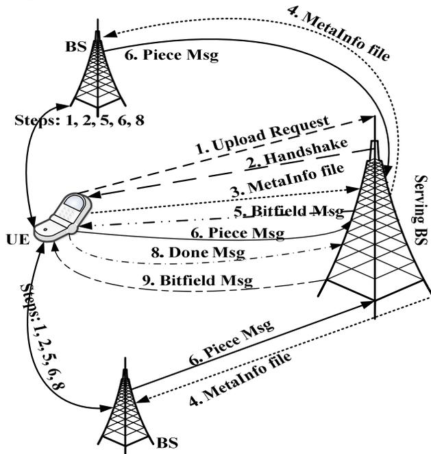
Figure 3. Segmented Upload Algorithm Message Transfer
