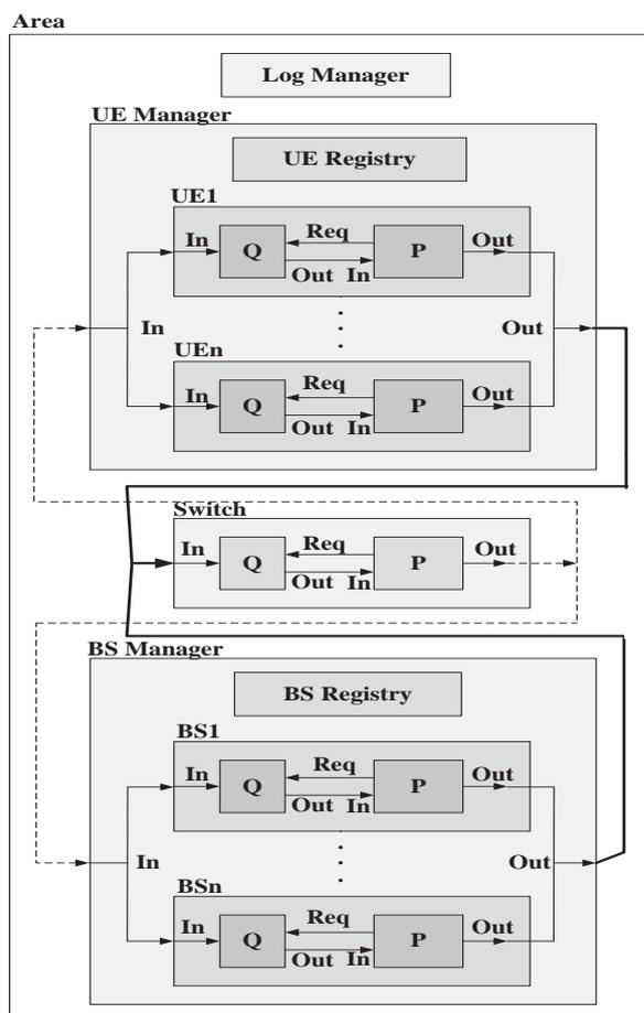
Figure 5. Simplified DEVS model hierarchy for a mobile network model (Q: Queue, P: Processor)
