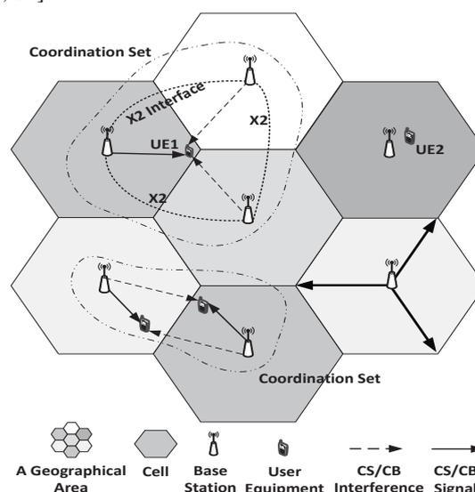
Figure 1. CS/CB transmission in LTE-Advanced
