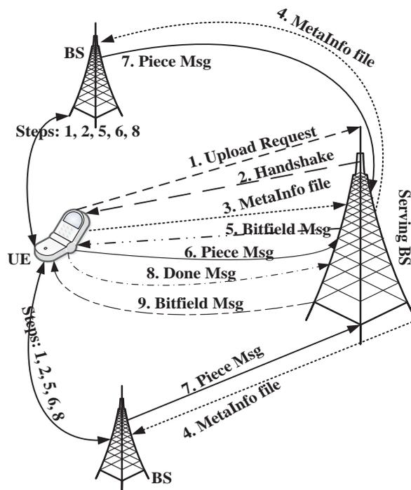
Figure 4. Segmented Upload Algorithm Message Transfer
