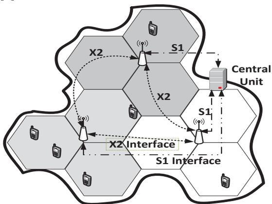
Figure 2. Centralized CoMP transmission in LTE-Advanced
