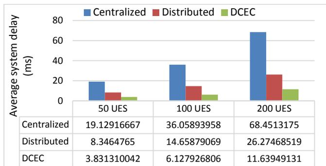
Fig. 9. Average system delay for 50, 100, and 200 UEs
