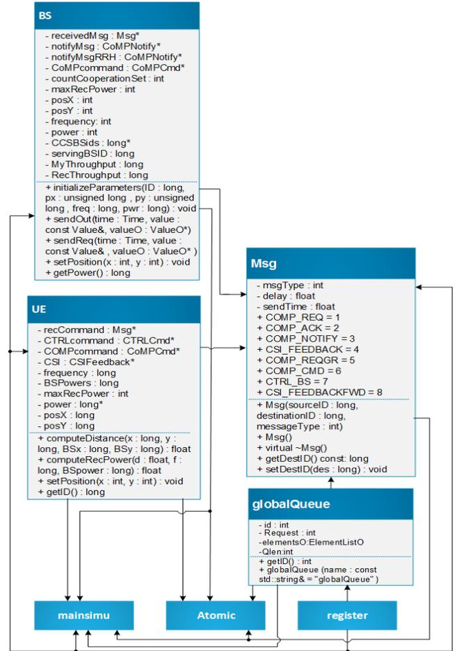
Fig. 3. Simplified class diagram of the model
