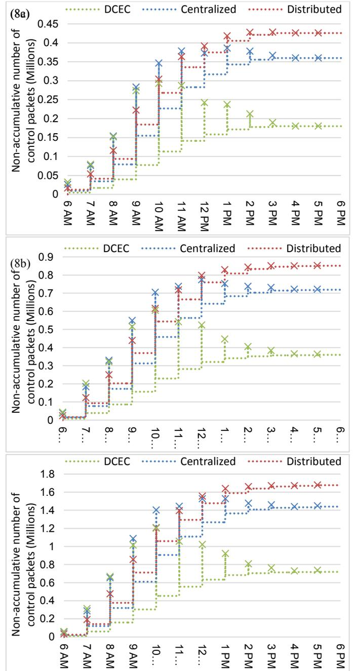
Fig. 8. Non-Accumulative number of packets for (a) 50, (b) 100, (c) 200 UEs
