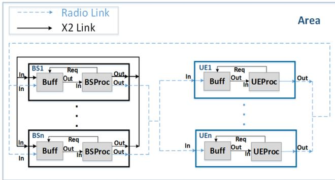
Fig. 2. Simplified DEVS model for CoMP control architecture
