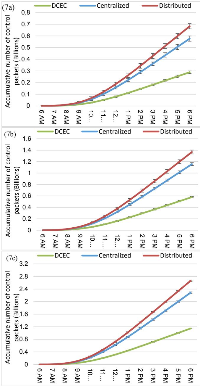
Fig. 7. Accumulative number of packets for (a) 50, (b) 100 UEs, (c) 200 UEs
