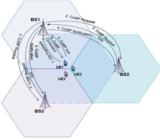
Fig. 1. Message transfer to elect CS and establish CoMP in DCEC-HetNet
