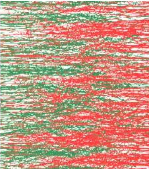
**Figure 5.** Trace of the emergent lane formation by virtual pedestrians simulated in a wide corridor.
