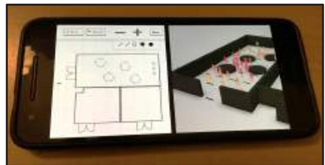
**Figure 13.** Demo of CPD running on Android; providing on-site scenario testing for event planners. It uses low-poly 3D character sprites, color-coded to indicate pedestrian density.
