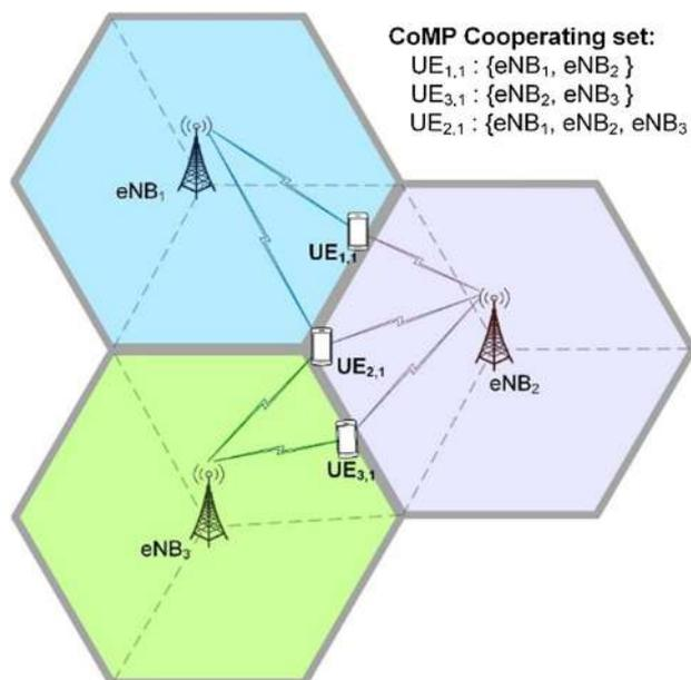
Fig. 6 A typical Multicell Cooperative Communication
