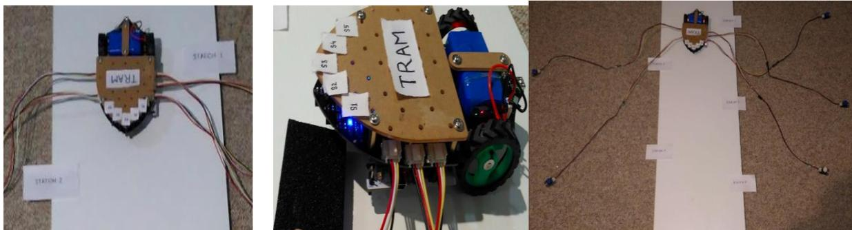
**(Left) The O-train positioned at station 1 waiting for a request. (Center) Next stop is requested through IR-sensor 1. (Right) Train Movement, different stations and their respective push buttons**
