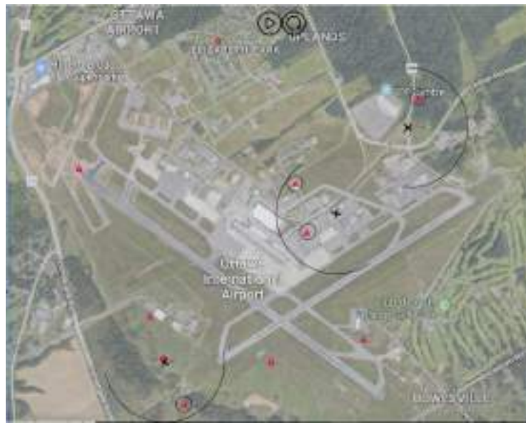
Fig. 2. Scenario 1: Test bed with 3 UAVs with short perception distance and 10 threats.
