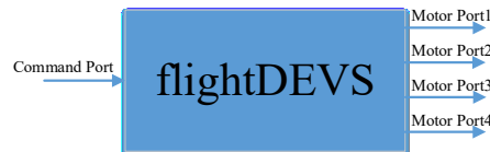
Figure 8. The flightDEVS atomic model.
