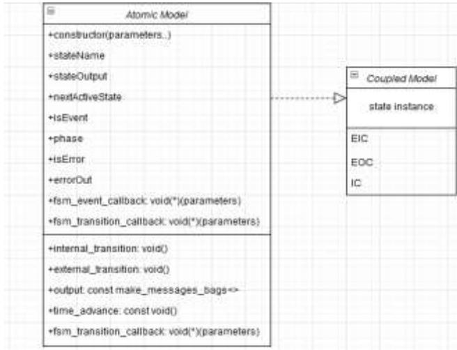
Figure 2: Class Diagram of the software model.
