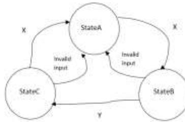
Figure 8: A simple Finite State Machine
