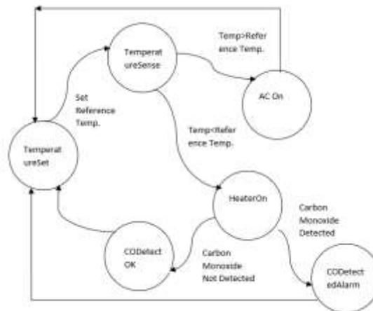
Figure 14: State Diagram of Automatic Temperature Controller
