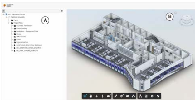
Figure 2. Forge Viewer user interface. (A) shows access to BIM 360 API, a repository for BIM models. (B) shows the rendering of the BIM model and default settings.
