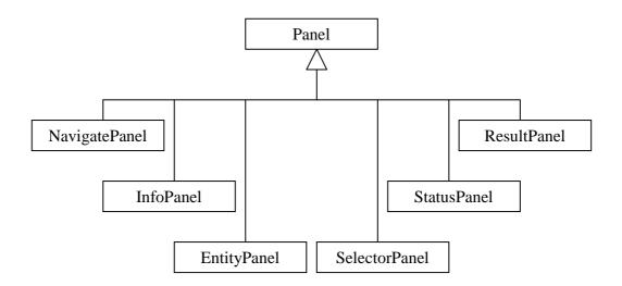
Figure 5.4 Class diagram of the classes extending Panel
