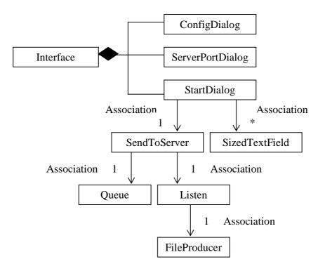
Figure 5.6 Class diagram of the client Interface
