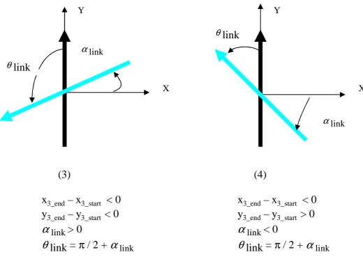
Figure 5.12 Calculate the rotation angle
