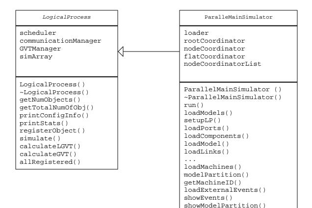
Figure 33: Classes LogicalProcess and ParallelMainSimulator
