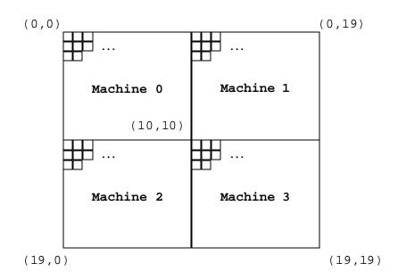
Figure 49: Partition of 20x20 life model in 4 machines
