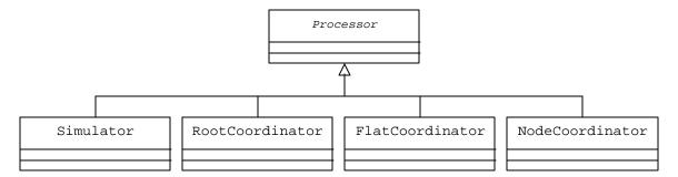
Figure 16: New processors' class hierarchy in CD++
