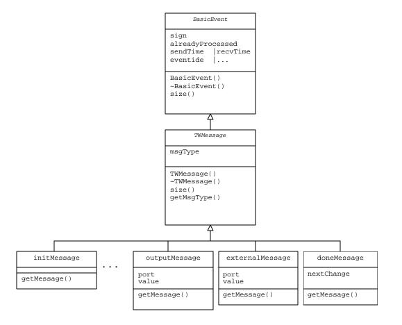
Figure 32: Class diagram for messages in CD++
