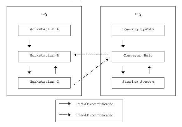
Figure 11: Automated Manufacturing System partitioned in two LPs
