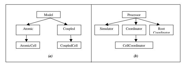
Figure 4: CD++ (a) Model hierarchy, (b) Processor hierarchy
