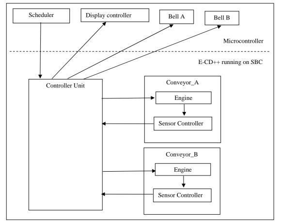
Figure 36 Hybrid AMS Scheme (scheduler, display and bells in hardware)
