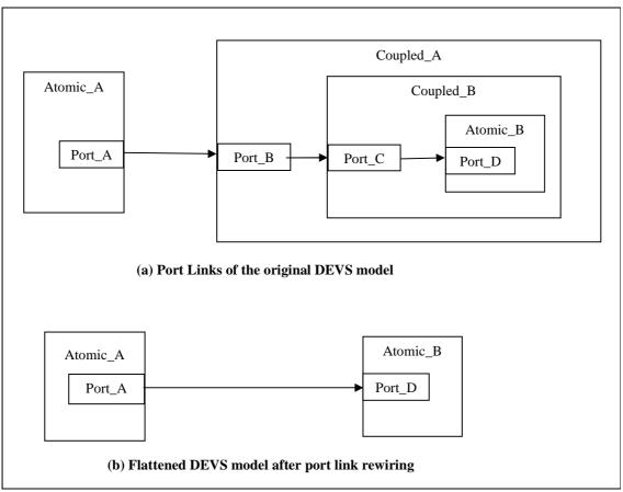
Figure 22 Port Link Rewiring by Flattened Coordinator Technique
