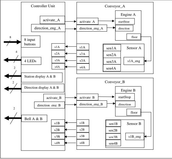
Figure 38 Modelling Scheme of the Simulated Part of AMS
