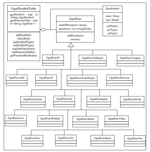
Figure 26 is the class diagram for GgadSymbolTable, GgadSymbol, and GgadFunc.
