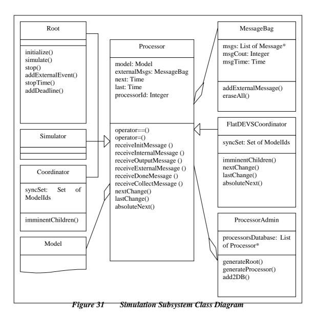
Furthermore, the Processor class defines the prototypes of handlers that respond to various DEVS messages, including initialization, internal and external state transition, output, collect and done messages. These methods in the Process class, however, are pure virtual functions which will be overloaded by the Simulator and Coordinator class.
