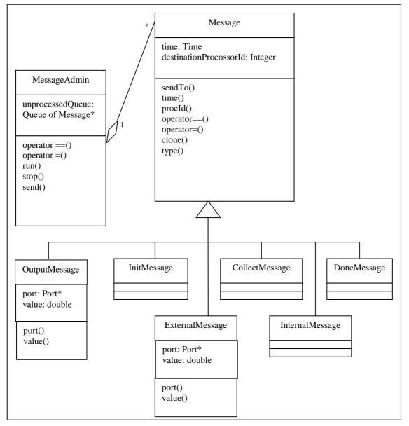
Figure 32 Messaging Subsystem Class Diagram
