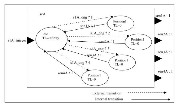
Figure 39 GGAD Graphical Notation of the Sensor Controller
