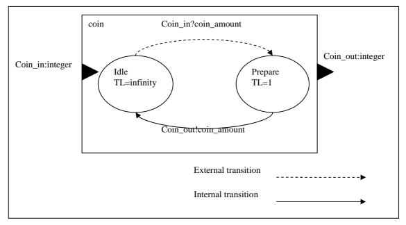
Figure 4 Graphical definition of an atomic model: Coin Displayer
