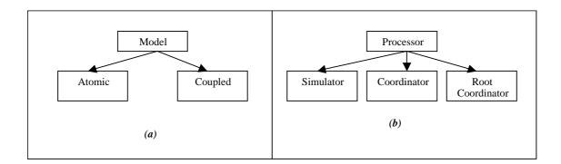
Figure 3 CD++ (a) Model hierarchy, (b) Processor hierarchy
