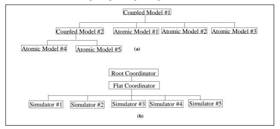
Figure 15 Flattened Coordinator Technique (a) Example of a model hierarchy, (b) Associated processor hierarchy
