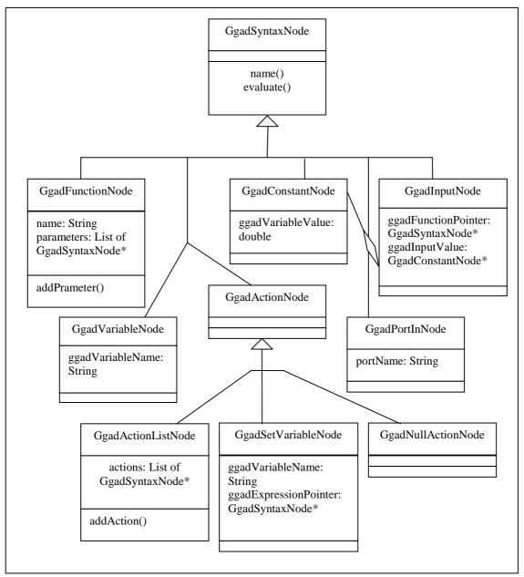
Figure 27 GGAD Syntax Tree Class Diagram
