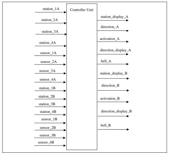
Figure 35 Diagram of the Controller Unit
