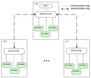
Figure 1. Hierarchical architecture of the first parallel CD++ simulator
