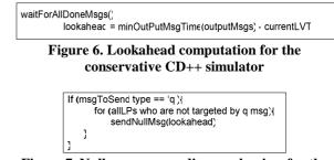
Figure 7. Null-message sending mechanism for the conservative CD++ simulator
