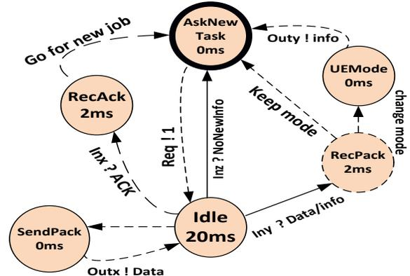
Figure 3. UE Processor DEVS graph
