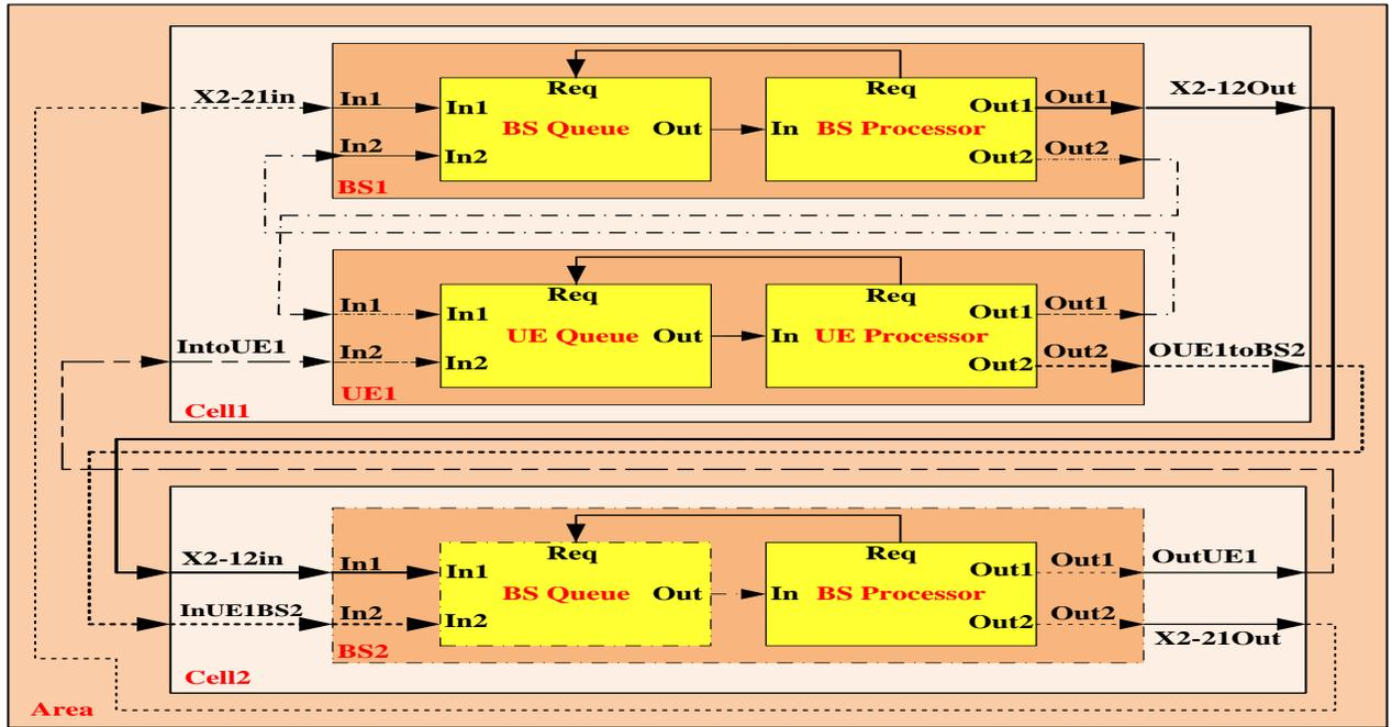
Figure 2. Simplified DEVS model hierarchy for mobile network model
