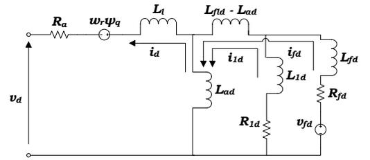
Fig. 2. d-axis synchronous machine equivalent circuit.
