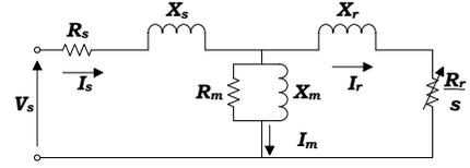
Fig. 1. Induction machine equivalent circuit.
