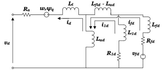
Fig. 3. q-axis synchronous machine equivalent circuit.
