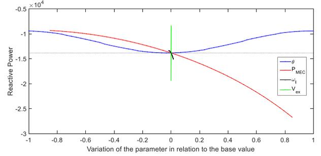
Fig. 6. Graph-spider of data simulated of power generation system for reactive power with the inductive synchronous generator.
