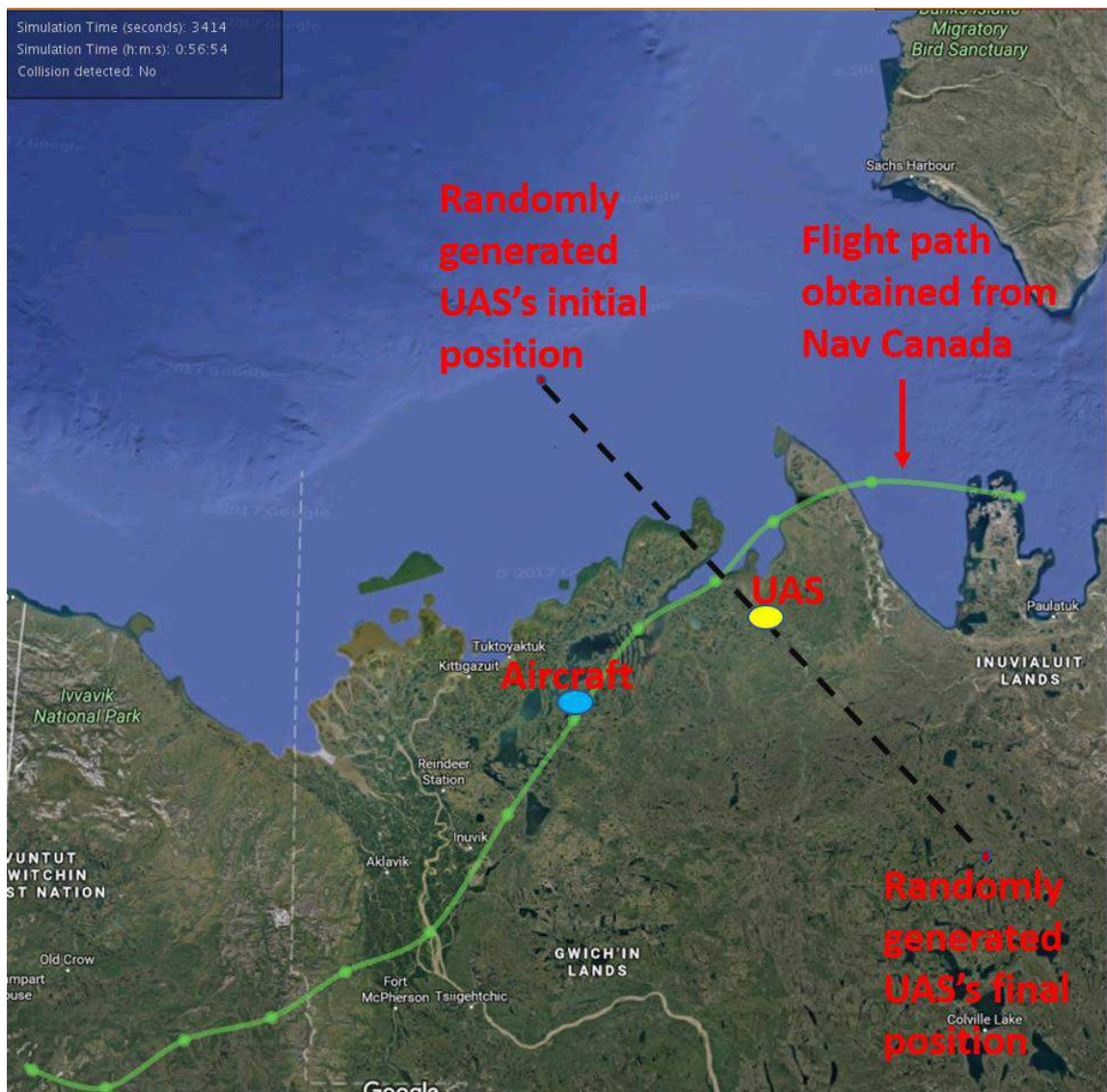
Figure 19: Snapshot of the Display Window (with annotations) taken while the UAS model was running
