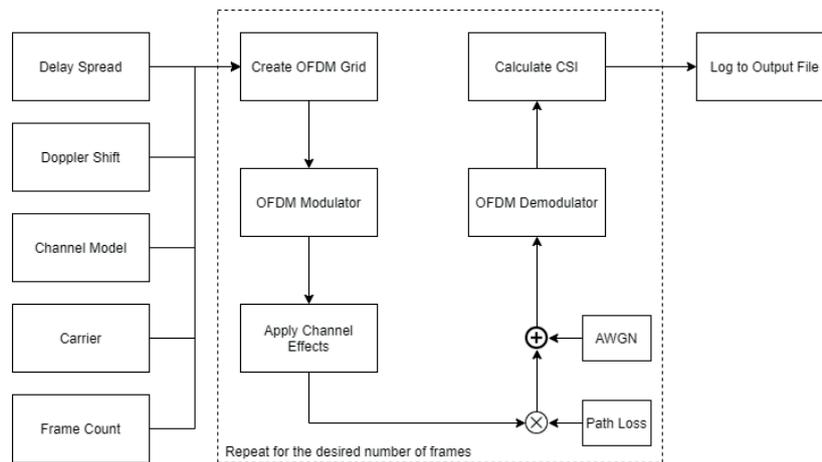
Figure 1: Simulator Block Diagram.
