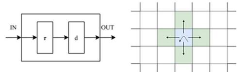
Fig. 1. Cell-DEVS model: (a) Atomic cell schematics; (b) 2-dimensional Cell-DEVS neighborhood
